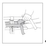
Secure the locking clasp. A click is heard when the clasp locks into place. Now, transfer the patient with the VanTurn. Plan the setting so as to minimize transfer time.
